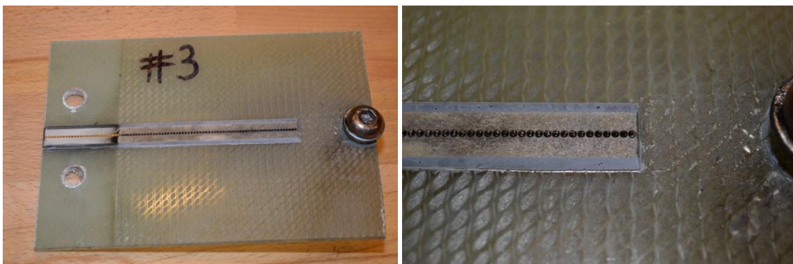
Figure 4 – Sample 3 after all three tests, with all buttons intact.
